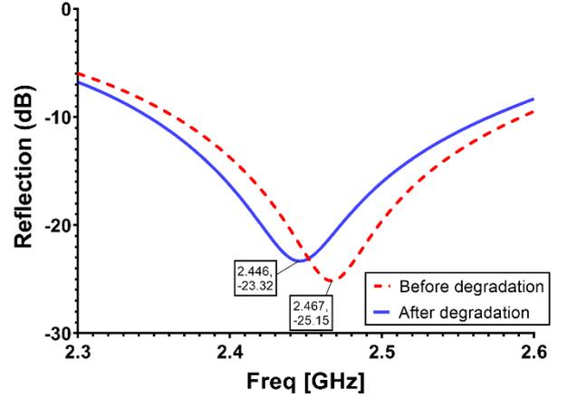
Fig. 4. The |S11| of the on-body reader antenna
