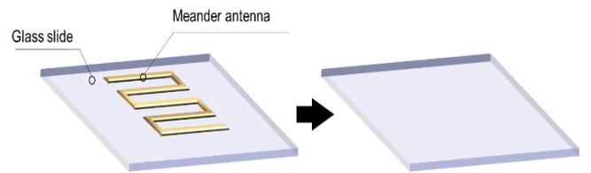
Fig. 2. Schematic representation of in-body reflector antenna before and after degradation.
