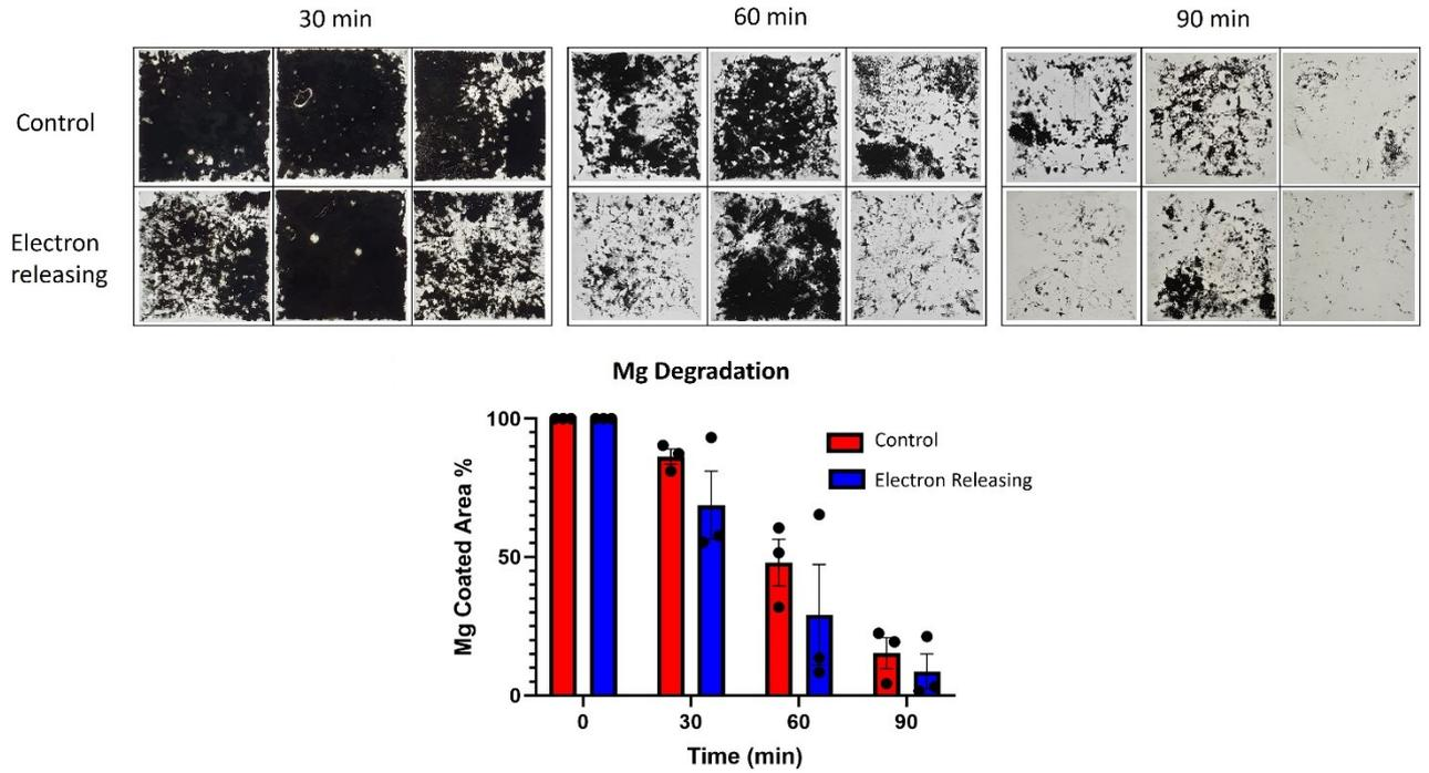
Fig. 1. Bacterial degradation of Mg-coated coverslips and graphical representation of decrease in Mg-coated area depict the decrease in Mg-coated area in. Mg biodegradation occurs faster with engineered bacteria expressing electron conduit proteins. According to the vision mapped here, the degradation speed will be linked to the arrival of the molecule of interest
