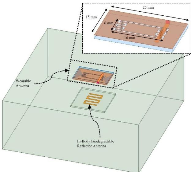
Fig. 3. HFSS model of the overall setup
