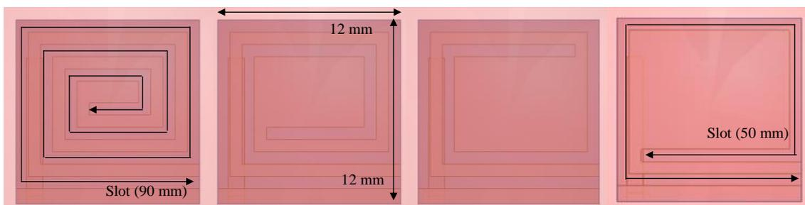
Figure 1 Implantable cavity backed meandered slot antenna (12 mm x 12 mm x 1 mm): the slot length is changed between 90 mm and 50 mm from left to right.
