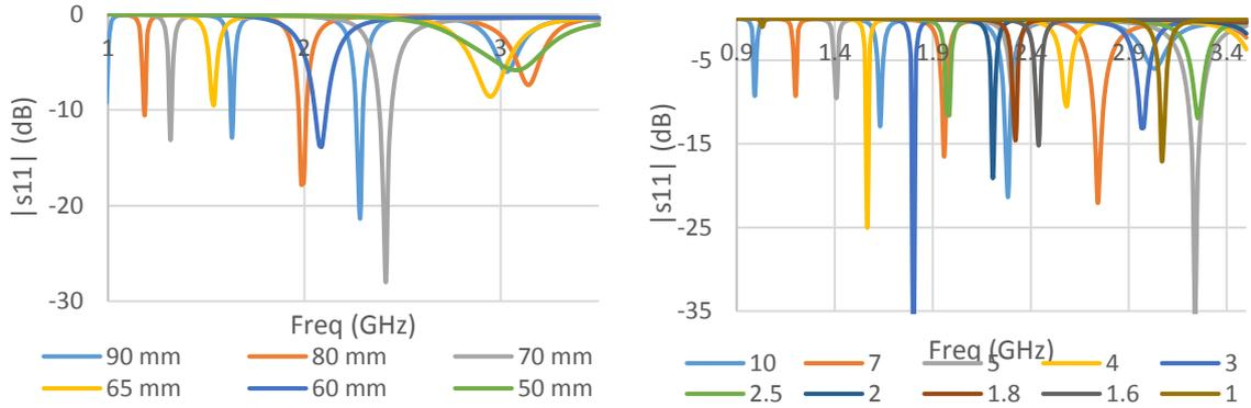
Figure 2 The frequency response of the cavity backed meandered slot antenna as the slot length is changed (left), and as the relative permittivity is changed from 1 to 10 (right).
