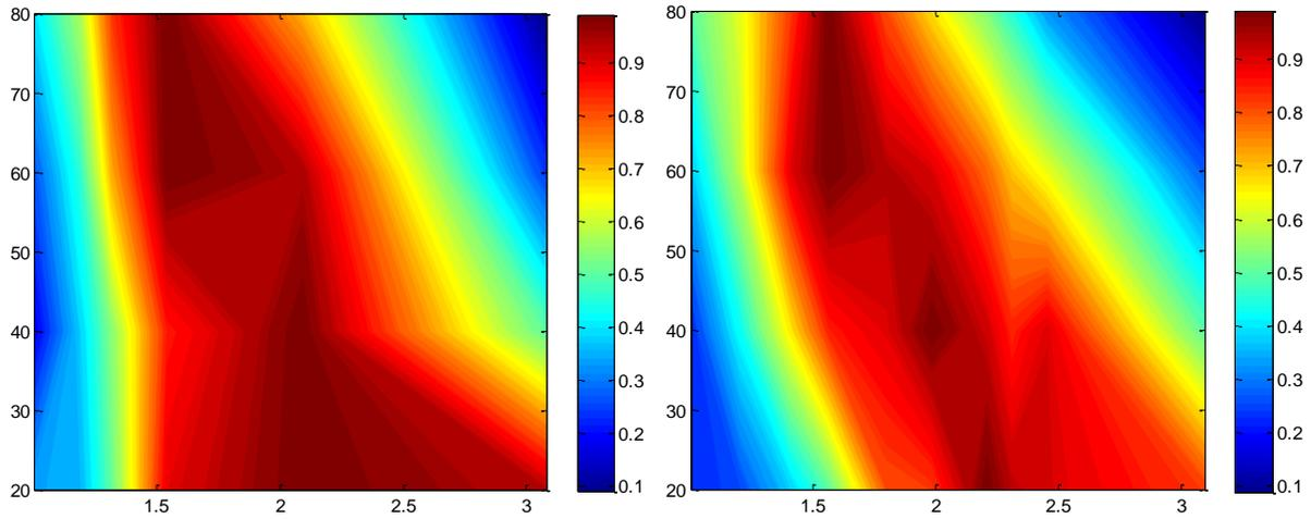
Figure 5 Normalized Maximum Poynting vector values plotted against depth and frequency, frequency of operation is changed by slot resizing and dielectric loading
