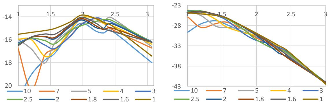
Figure 4 Radiation efficiencies of the antenna set tuned with dielectric loading merged into 20 mm and 80 mm radius of muscle spheres
