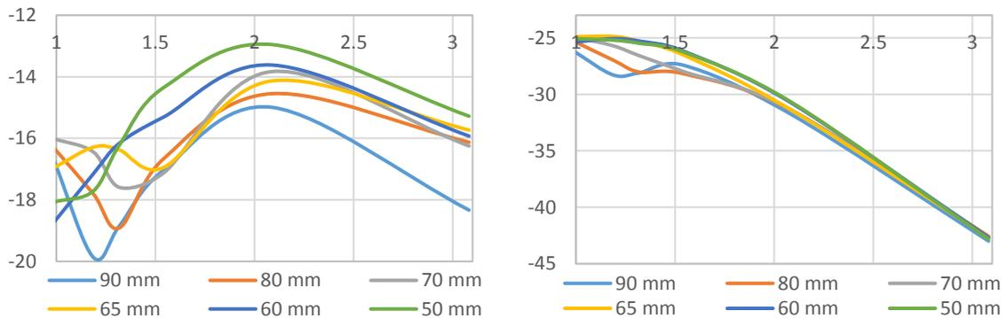
Figure 3 Radiation efficiencies of the antenna set tuned with slot resizing merged into 20 mm and 80mm radius of muscle spheres
