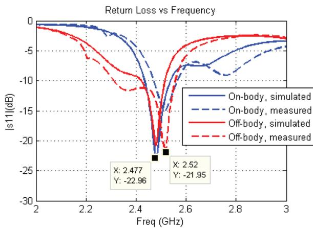
Fig. 3.  $|s_{11}|$  vs. frequency of the proposed antenna with 100 MHz Bandwidth for the off-body mode and 120 MHz Bandwidth for the on-body mode
