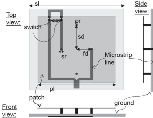
Fig. 1. Top, front and side view if the proposed dual mode antenna which comprises a switching mechanism to switch between two radiation modes: horizontally omnidirectional and broadside radiation
