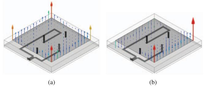
Fig. 2. Vector E field distributions of  $TM_{00}$  (a) and  $TM_{01}$  (b) modes which support on-body and off-body operations respectively
