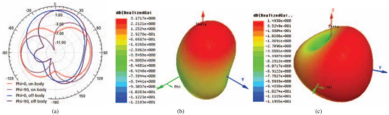
Fig. 4. Radiation patterns of different modes of the antenna in isolation at the resonant frequency: Fig.4(a) 2D Radiation Pattern of each mode at  $\phi=0$ , Fig.4(b) 3D Radiation Pattern of the off-body mode, Fig.4(c) 3D Radiation Pattern of the on-body mode
