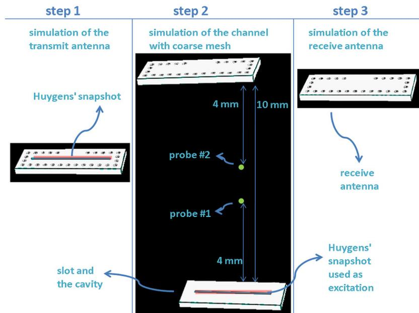
Fig. 8 The three steps of the channel simulation with Huygens' Technique, 1<sup>st</sup> step: simulation of the Tx antenna with fine mesh, 2<sup>nd</sup> step: simulation of the whole scenario with coarse mesh, 3<sup>rd</sup> step: simulation of the Rx antenna with fine mesh.
