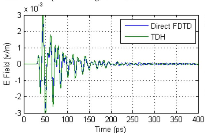
Fig. 4 Verification of the Huygens' technique at step 2, E field variations at Probe #1
