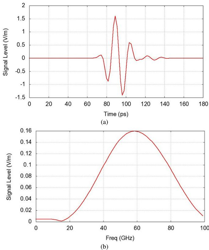
Fig. 3 The excitation waveform in time (a) and frequency (b) domains
