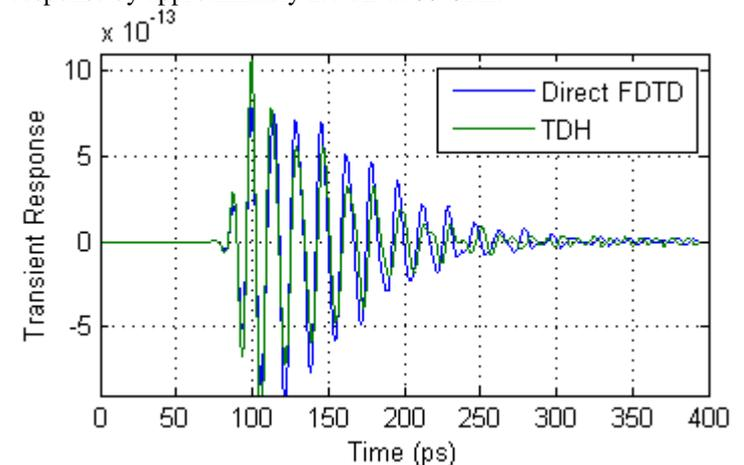
Fig. 6 The transient response as seen in the receive antenna obtained with Huygens' Technique and direct simulations
