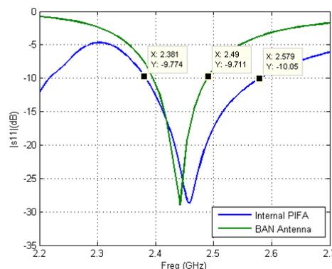
Fig. 2. Comparison of s11 for internal PIFA and BAN antenna
