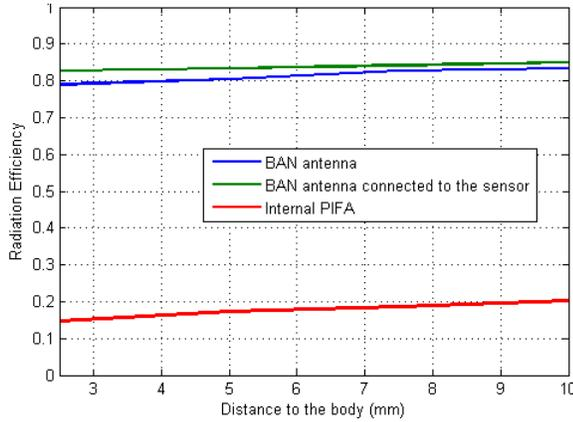
Fig. 6. Effect of antenna body separation on the radiation efficiency
