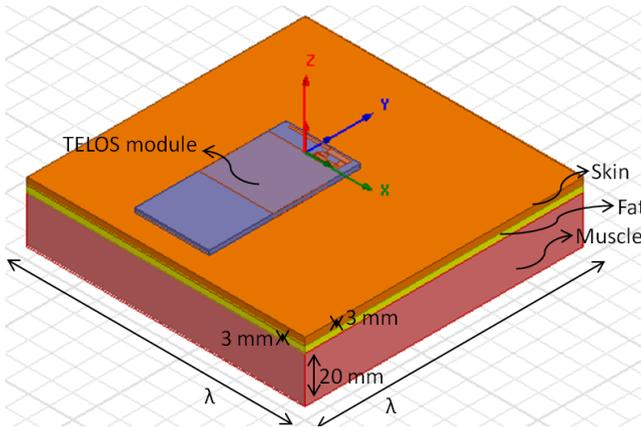
Fig. 4. Numerical layered planar phantom for human chest
