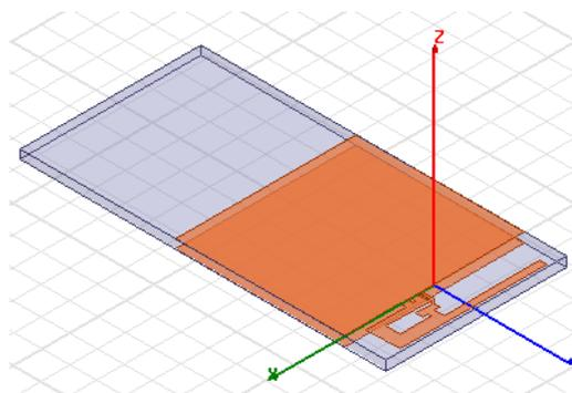
Fig. 1. Internal PIFA modelled in HFSS
