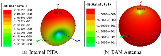
Fig. 3. 3D Radiation pattern of the antennas in Isolation
