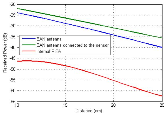
Fig. 7. Received power at 2.35 GHz vs different transmitter receiver separations
