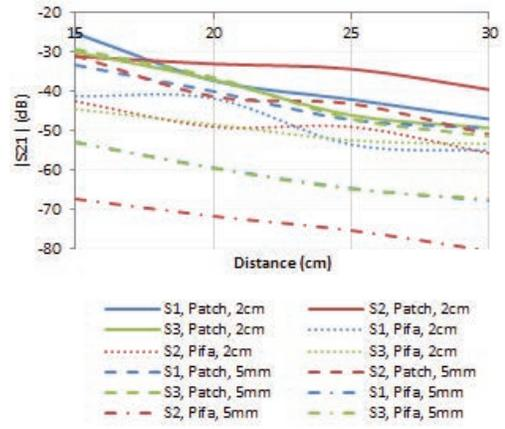
**Figure 4: ARB Propagation: Back to back transmission versus path length for 5mm and 2cm antenna-body separations for the Patch antenna and the internal PIFA of the TelosB mote, where “S1, S2 and S3” are the subjects**
