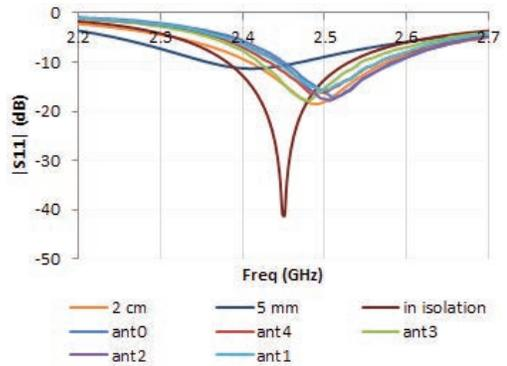
Figure 2: Simulated frequency response of the antenna on a three layered planar phantom connected to the TelosB mote for  $5mm$  and  $2cm$  antenna body separations and Measured frequency responses of the rectangular shorted patch antenna demonstrating the repeatability of the structure
