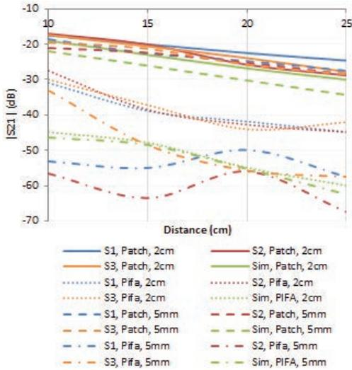
**Figure 3: ALB Propagation: Back to back transmission versus path length for 5mm and 2cm antenna-body separations for the Patch antenna and the internal PIFA of the TelosB mote, where “S1, S2 and S3” are the subjects and “Sim” stands for HFSS simulations**
