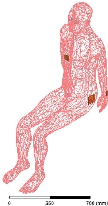
Fig. 1. Wearables simulated on ANSYS human body phantom, Male-4mm accuracy
