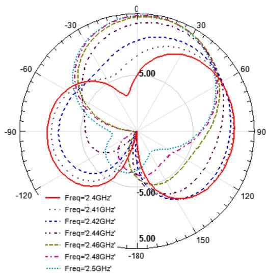
Fig. 4: 2D demonstration of the beam steering: Gain pattern in dB at  $\phi=0^\circ$  at 6 frequency points
