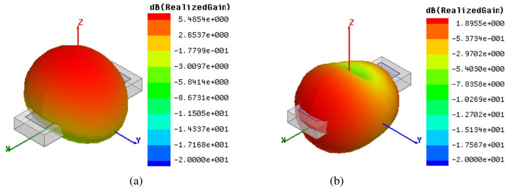
Fig. 3: (a): 3D Gain pattern of the azimuth mode in linear scale at 2.4GHz corresponding to channel 11 in Zigbee, (b): 3D Gain pattern of the elevation mode in linear scale at 2.48GHz corresponding to channel 26 in Zigbee
