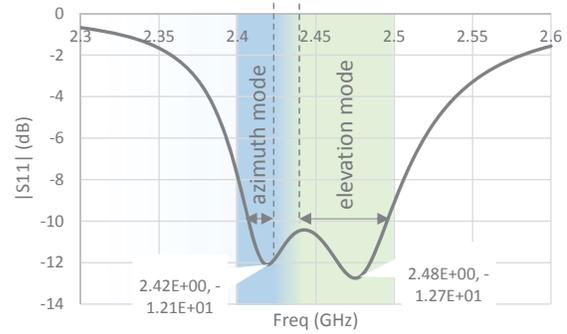
Fig. 2:  $|s_{11}|$  vs. frequency: 85 MHz 10 dB bandwidth from 2.395 GHz to 2.48 GHz, centre frequency of the azimuth mode and the elevation mode at 2.42 GHz and 2.48 GHz respectively
