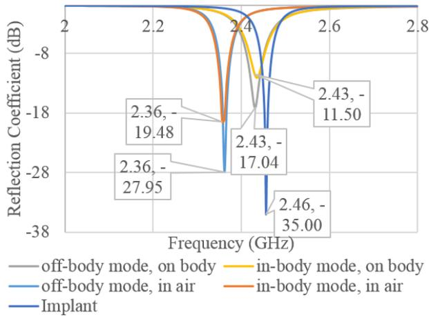
Fig. 2: The  $|s_{11}|$  of the repeater antenna for each activation: in-body mode and off-body mode when the antenna is located in air and on a tissue block with 4 cm separation between the skin and the antenna, and of the implant antenna of the test scenario.
