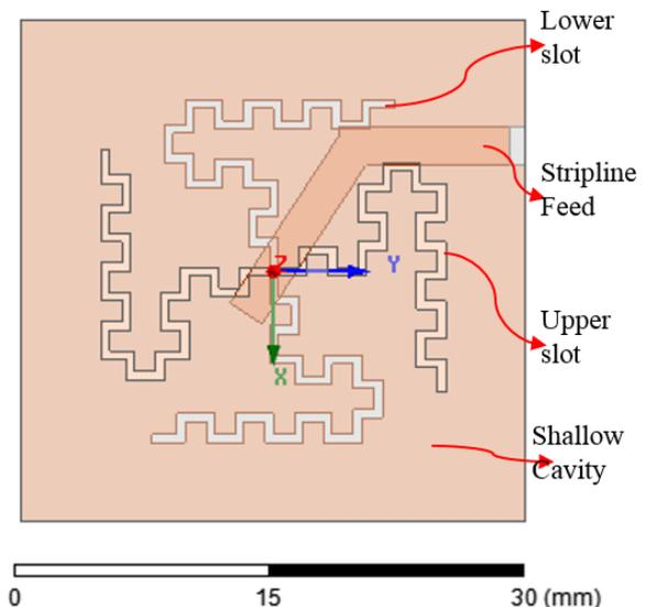
Fig. 1: Antenna diagram, slots miniaturized inspired by second order Koch-fractal configuration
