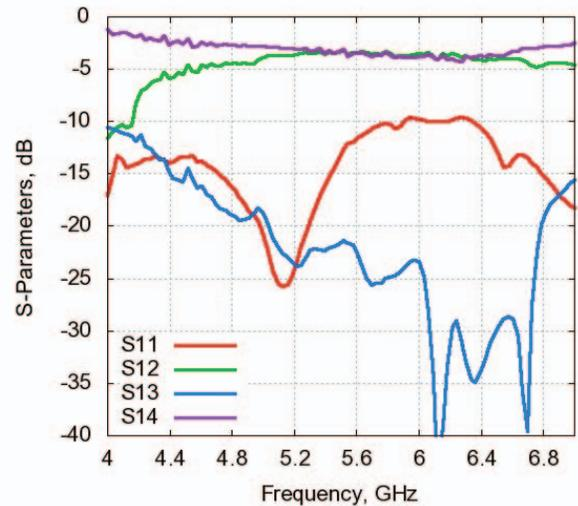
Figure 4 Measured S-Parameters of the Hybrid
