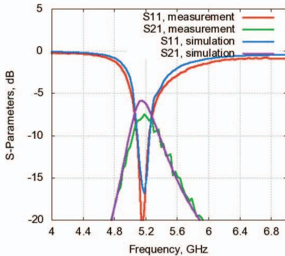
Figure 2 Measured and Simulated S-Parameters of the array before decorrelation
