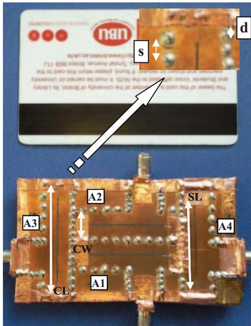
Figure 1 4 element array, where CL: cavity length, CW: cavity width, SL: slot length, s: shoring pin separation, d: shoring pin diameter
