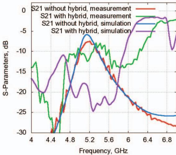
Figure 6 Simulated coupling between the closely spaced antenna elements
